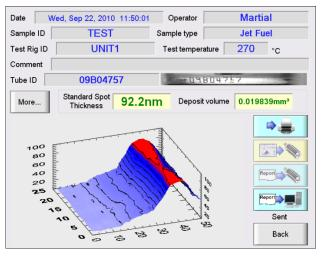
Until 2014, only the visual rating method was used for specification purposes but it was suffering from the drawback of operator subjectivity. ASTM decided to use SI unit to report the result of the jet fuel thermal oxidation deposit. Following this decision, the DR10 – ITR became referee method.
