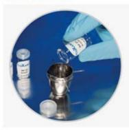
The customer receives a glass powder that contains a standard and flux. By directly filling the powder into the platinum crucible, a glass bead can be melted as a calibration standard for XRF without accurate weighing.
