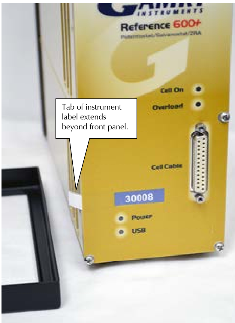
Figure 4-6 Removing the Front Bezel
