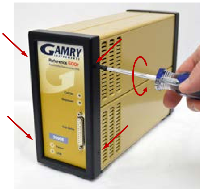
Figure 4-5 Removing the Front Bezel
