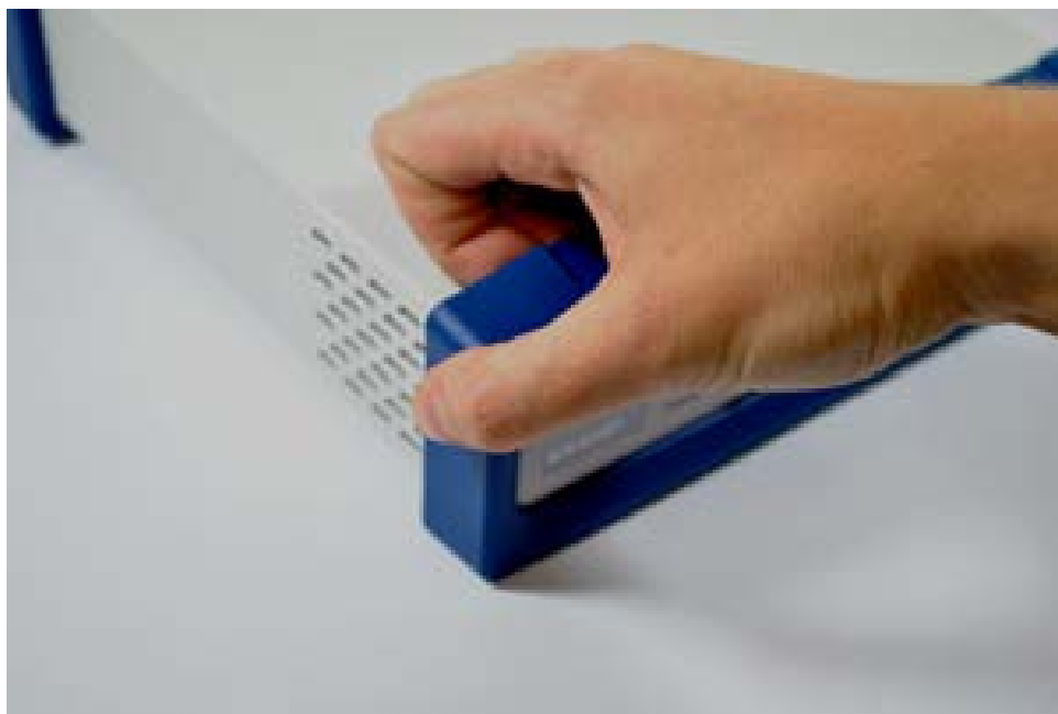
Figure 3-4 Removing the Front Bezel
