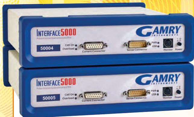
The Interface 5000 is designed for testing of batteries, supercapacitors, and fuel cells. There are two versions available, the 5000P which provides capabilities for typical testing of single cells using techniques such as charge, discharge, cyclic charge/discharge, potentiostatic, galvanostatic, and galvanostatic EIS to 20 kHz. The 5000E includes Gamry's full suite of electrochemical techniques and extends the impedance frequency range to 1 MHz.
